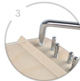
Tighten the tuning pin approximately five complete turns. Be sure that the string is being wound below the hole in the tuning pin.
